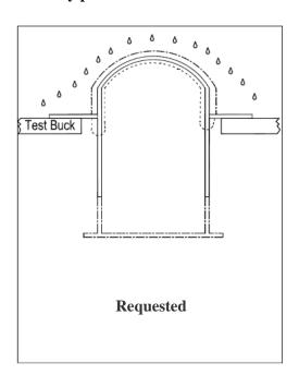
Plane of Measured Air Leakage
